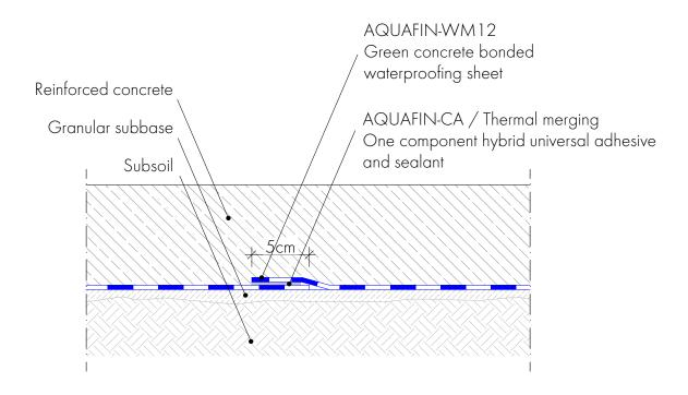
Overlap area thermal merging / bonding >4cm
