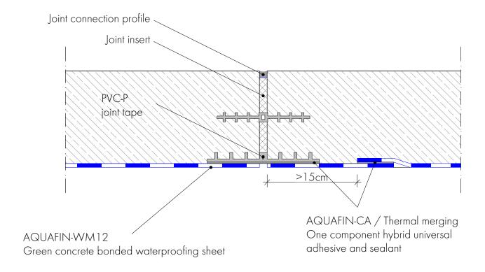
Thermal merging / bonding in the overlapping area >4cm
